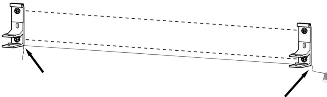
10) Slide the awning (cassette) on wall brackets so that the construction is maximally pressed to the back (Note – before placing the awning verify the alignment of brackets – wall surface should be of the same thickness at installation spots).
