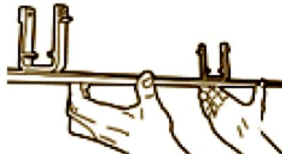
16) Fasten the masking frame profile with brackets to the square bar 40x40 using M8x70 screws.
